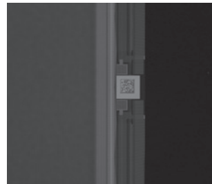
Phone inner screen 2D code detection
