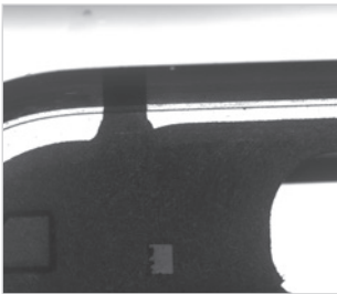
Phone frame inner dimension detection
