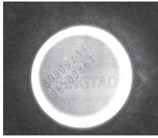
Production date detection on bottle caps
