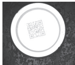
2D code detection on plastic caps
