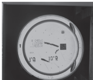
Piston defect detection and dimension detection
