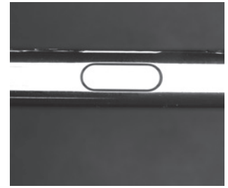
Phone charging port position detection
