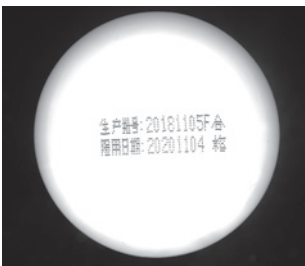
Production date detection at the bottom of cosmetic bottles
