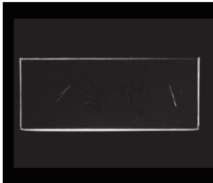
Cigarette package surface scratch detection
