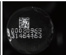
Invisible Code Detection on Bottle Cap
