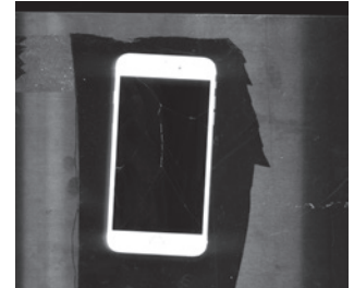
Phone screen scratch detection
