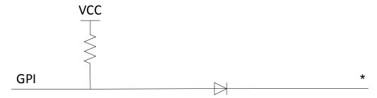
Figure 10-5 Internal Circuit of Non-Isolated Input
